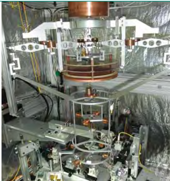
Mechanism of the BIPM watt balance under construction at the BIPM at Sèvres. (Reproduced with permission from BIPM.)
