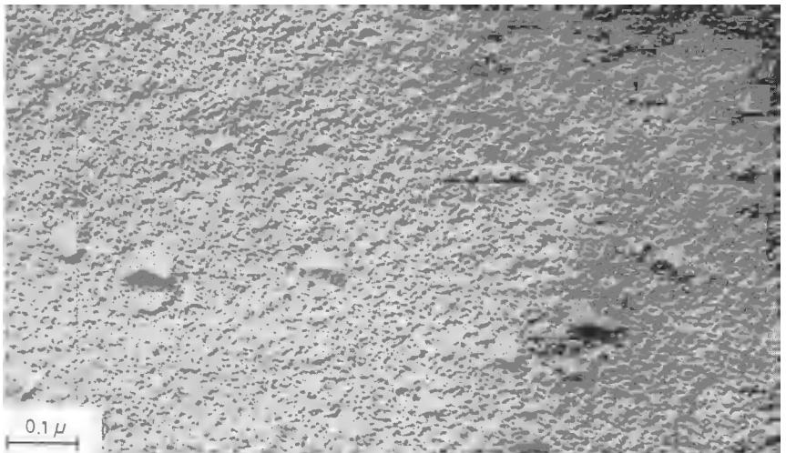
Figure 8. Thin film of atactic polystyrene stretched 100% on Mylar, Pt-shadowed.
