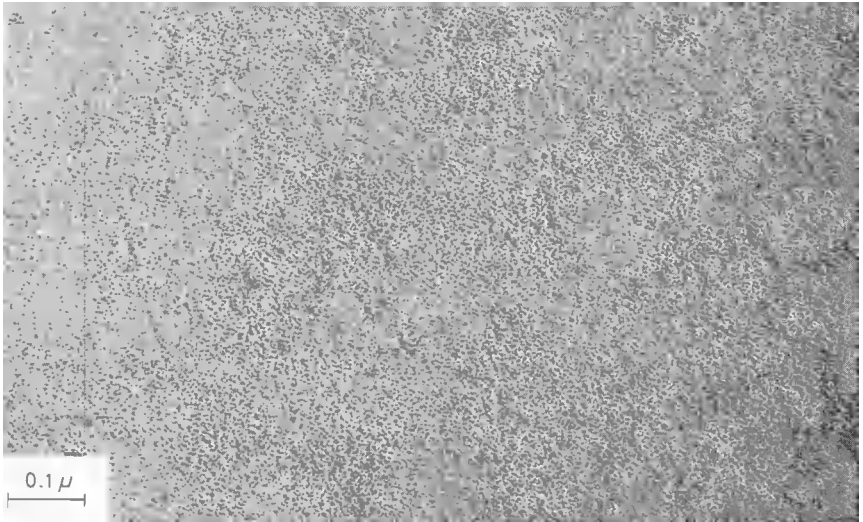
Figure 7. Unstretched thin film of atactic polystyrene, Pt-shadowed.
