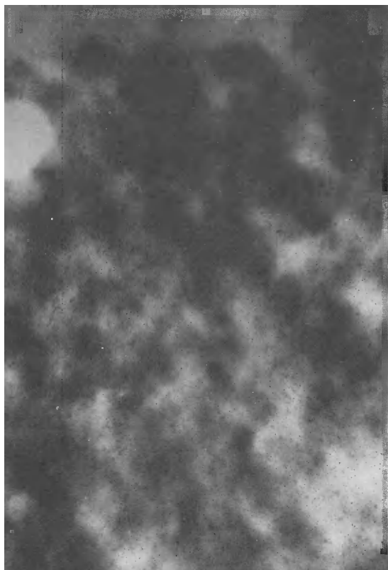
Figure 5. Electron micrograph of IPN-11 : 90/10 polyurethane (PU-9) and polystyrene; \times 75\,000 ; reduced to \frac{2}{3} on reproduction.
