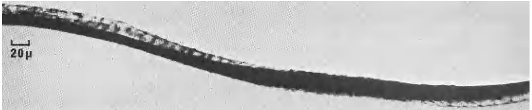
Fig. 12. Merino wool fibre stained with gold preferentially in the paracortex which forms the inside of the crimp wave. 34
