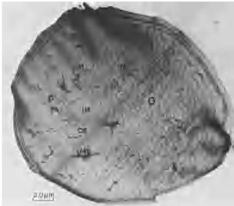
Fig. 9. Electron micrograph of a cross-section of a Merino wool fibre stained with phosphotungstic acid showing orthocortex (O), paracortex (P), macrofibrils (M), nuclear remnants (NR), cell membrane complex (CB) and intermacrofibrillar material (IM). 30
