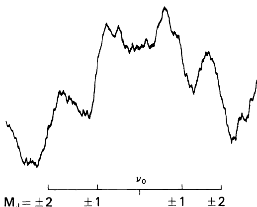
Fig. 3. The J = 3 + 2 transition of the SO radical in the ^1\Delta electronic state: Stark dc bias = 55.3\text{ V/cm} ; Stark ac modulation = 2.3\text{ V/cm} , \nu_0 = 127770.47\text{ MHz} .
