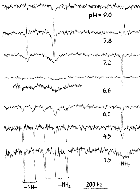
Figure 9. Natural-abundance ^{15}\text{N} spectra of 1.5 M arginine in water as a function of pH, protons coupled.
