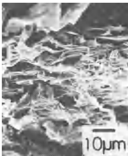
Fig. 4. Scanning electronmicrograph of fractured surface of a composite of PPTA microfibrils and PVC matrix prepared by casting the PVC solution in THF in which PPTA microfibrils are suspended.
