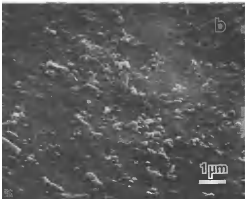
Fig. 1. SEM images of submicron particles in pond water. Specimens prepared by a) centrifugation and b) filtration
