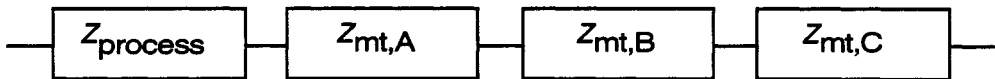
Fig. 5.1 Equivalent circuit representing the impedance due to a process involving three species A, B and C
