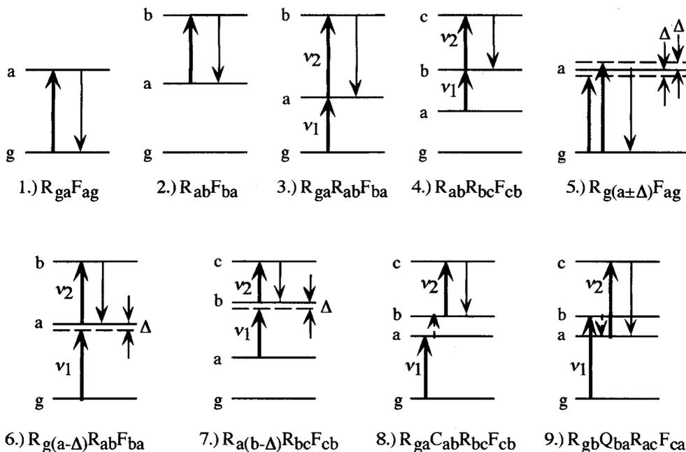
Fig. 3. Examples of resonance fluorescence processes
