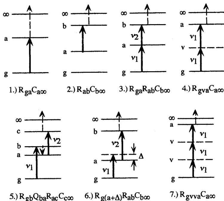
Fig. 7. Examples of laser enhanced ionization processes
