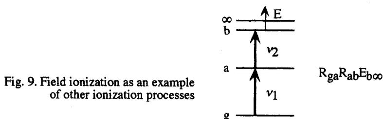
This process is usually named resonant, two-photon excitation, field ionization.
