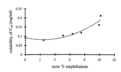
Dependence of solubility of  $C_{60}$  on the concentration of naphthalene in a) decaline; b) toluene; c) dodecane solvent mixtures
