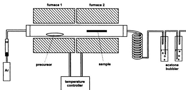
**Fig. 2** Pyrolysis set-up.
