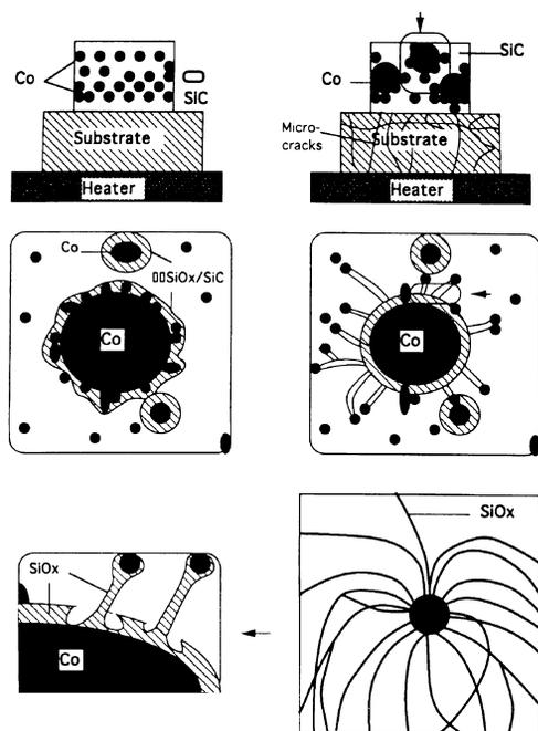
**Fig. 9** Nanoflower growth model: (a) Heating assembly; (b) Fissured  $\text{SiO}_2$  and agglomerated Co; (c) Spherical Co particles; (d) Initial growth stage; (e) Magnified nanotube growth; (f) Final stages of growth.
