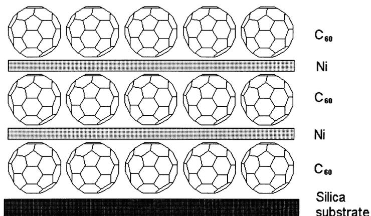
**Fig. 10** Thin layers of successively deposited pure Ni and  $\text{C}_{60}$ .
