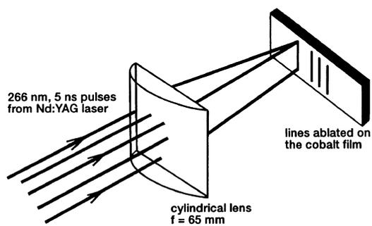
**Fig. 1** Laser etching set-up.
