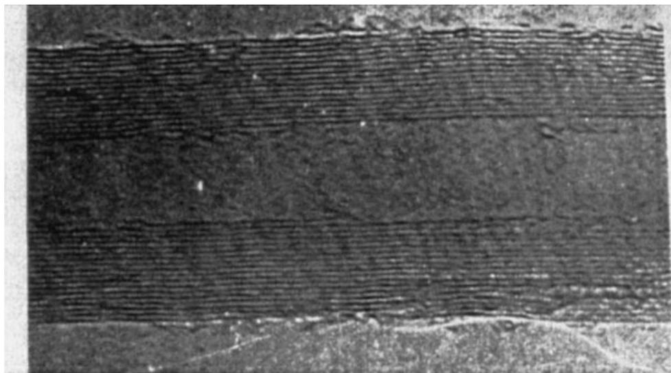
**Fig. 6** High resolution transmission electron micrograph showing the degree of graphitisation of an electrolytically formed multi-walled carbon nanotube. The interlaying spacing of the graphene sheets is 0.34 nm.
