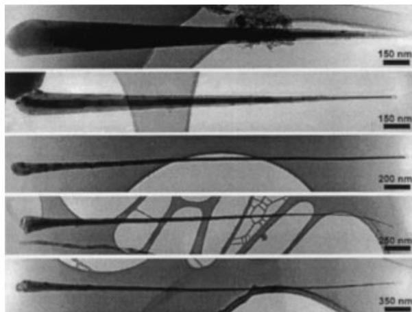
**Fig. 11** TEM images of five representative needle-like structures which were almost completely filled with Ni.
