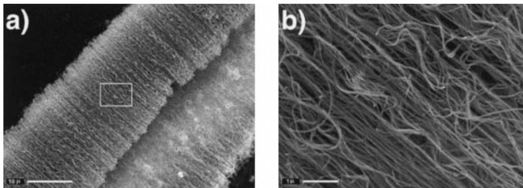
**Fig. 3** (a) SEM images of aligned nanotube films grown on Co-etched substrates using amino-dichlorotriazine as the organic precursor. (b) Close-up of 3a.
