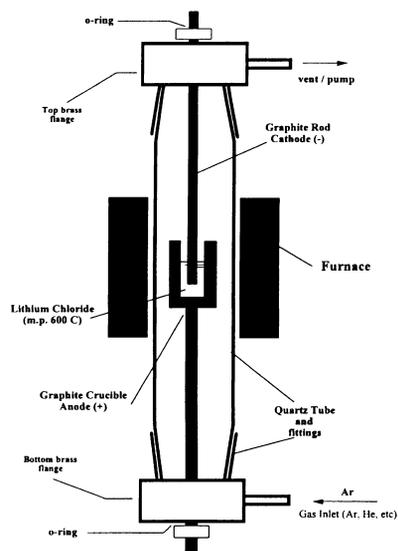
**Fig. 4** Electrolysis set-up.
