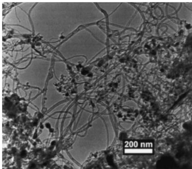
**Fig. 5** Low resolution transmission electron micrograph of electrolytically produced carbon nanotubes.
