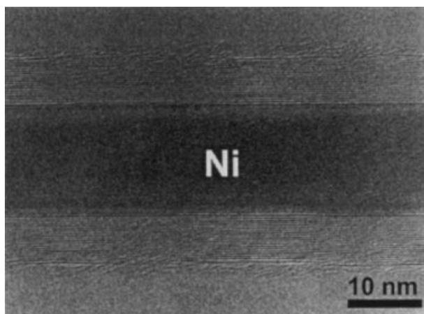
**Fig. 12** HRTEM image of a highly graphitised Ni-filled carbon nanotube. The quality of graphitisation is unusual for pyrolytically grown materials.
