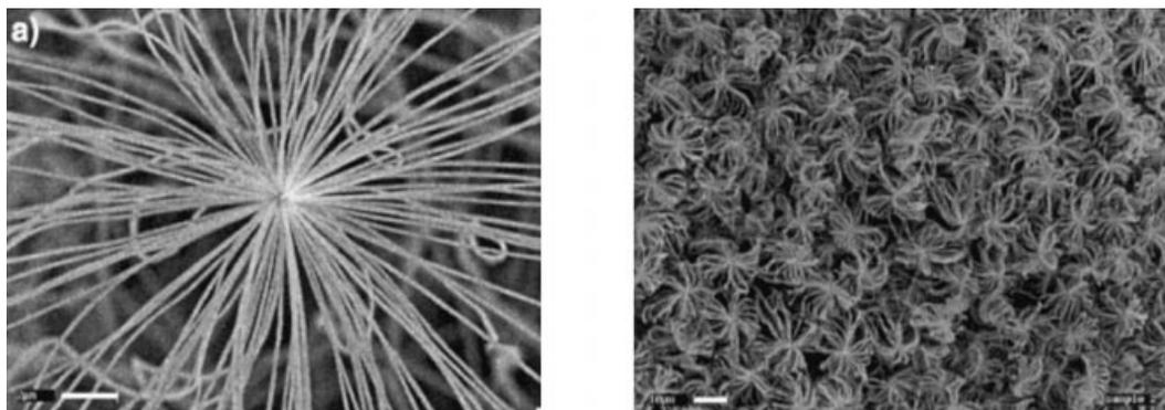
**Fig. 8** (a) SEM image of a single silica nanoflower exhibiting radially attached fibres to a central sphere. (b) SEM image of a silica nanoflower film produced in the presence of CO.
