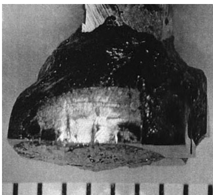
Fig. 15 Single crystals of neodymium barium cuprate grown by the modified Chokhralsky method from peritectic melts for the production of new generations of substrate materials for superconducting thin film in modern microelectronics.
