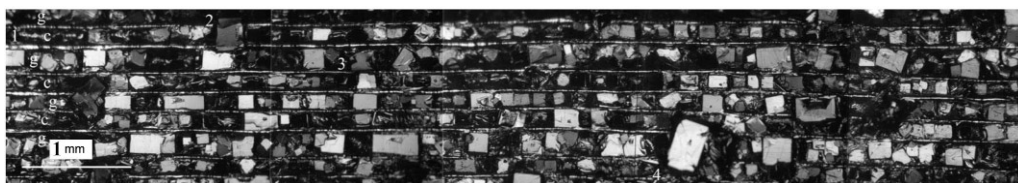
Fig. 14 Graphotexturing of HTSC cuprate to produce long-length conducting samples. About 200 crystals are well oriented between walls along a distance of 8–9 mm (as evident from their crystal habit). White stripes are silver-alloy walls.
