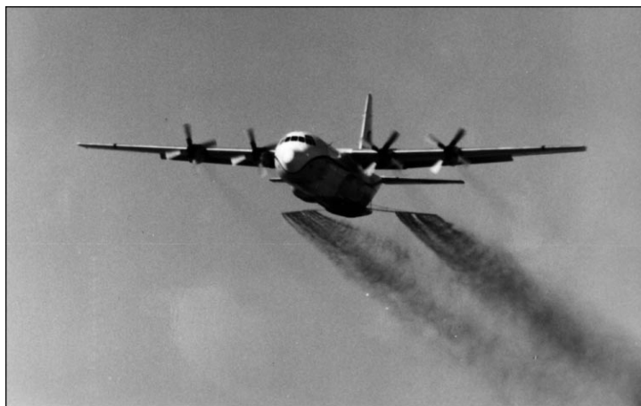
Fig. 3 C-130 with ADDS-Pack spraying dispersant.
