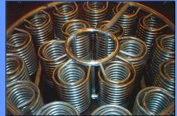
oil-steam heat exchanger
